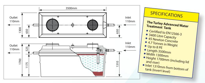
Turley's waste water treatment system tanks are durable and easy to install and can be utilised in those areas where the percolation area of the septic system does not meet the filtration requirements in terms of soil porosity.
