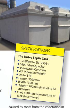
caused by roots from the vegetation in the vicinity and the acidity of the sewage. The Turley Septic Tank is designed with access covers, ten millimetre steel loops for handling, ventilation access, bitumen seal and pipe seal facilities at the inlet and outlet ends, is an ideal choice for not only new installations, but also is the tank of choice for replacement or upgrading of an existing tank.
